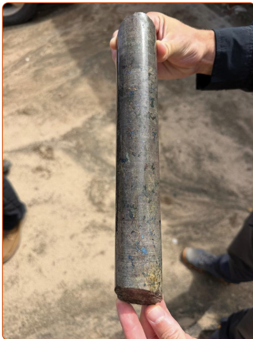
Figure 2. Newly discovered Margarita Skarn, Hole PH2-3, 628.79 to 629.80 metres: 2.10% Cu, 4.98 g/t Au, 35.0 g/t Ag. Bornite, chalcocite, covellite and chalcopyrite.
