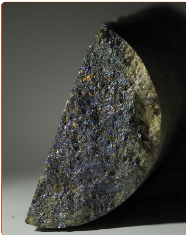
Figure 1. Hole PH2-3, sample 217671 (212.40 to 212.95 metres): 16.6% Cu, 1.1 g/t Au, 583 g/t Ag. Semi-massive chalcocite, bornite and chalcopyrite.
