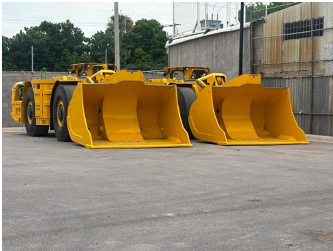
Figure 2: Contractor Scoop trams
