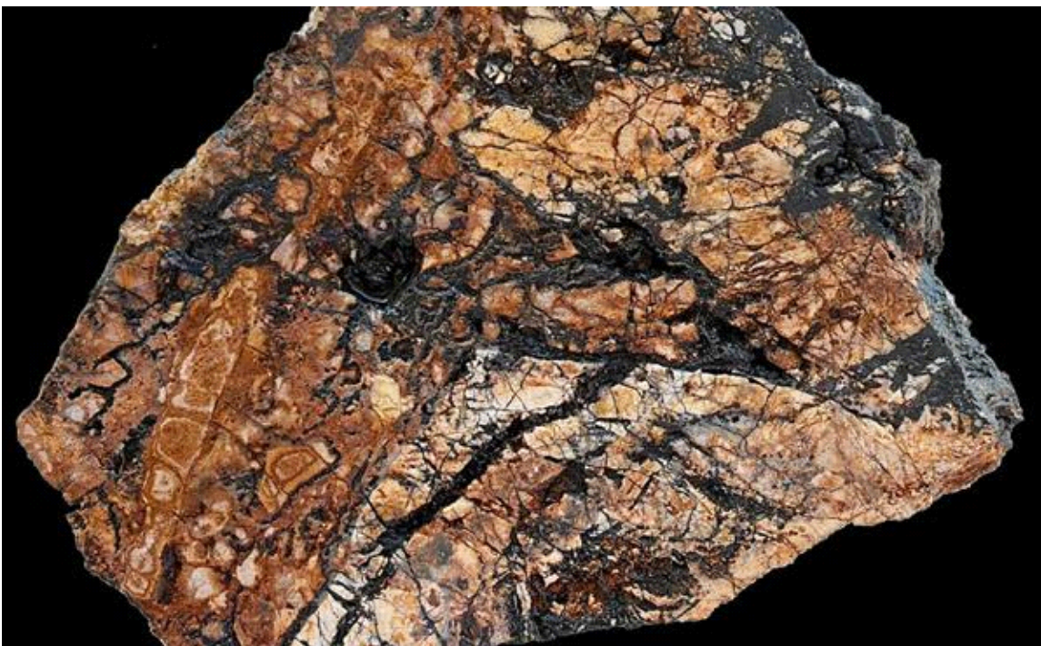
Figure 3: Brecciated, pervasively silicified and bleached tuff, with abundant hematite staining and hematite-goethite fracture fill. The sample is approximately 12 cm wide. Sample ON2-091.
