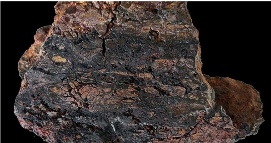
Figure 4: Hematite stained, multiphase quartz veins with abundant boxwork hematite and goethite after sulphides and hematite-goethite fracture fill. The sample is approximately 12 cm wide. Sample ON2-222.
