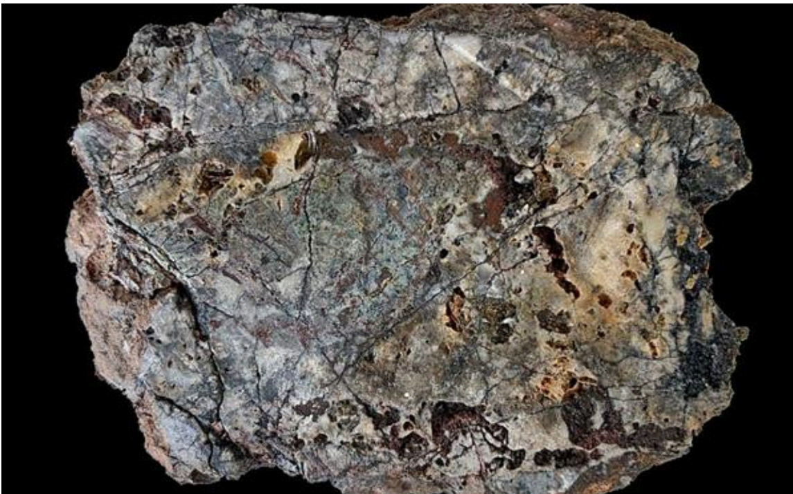
Figure 5: Saccharoidal vein quartzes with possible silicified and sericite-chlorite altered remnant wall rock clast. Note blebby iron oxide and iron oxide boxworks after sulphides. The sample is approximately 10 cm wide. Sample ON2-067
