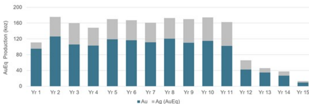
Figure 1: Annual production is forecast to average 134 koz AuEq over 14.4 years including 161 koz AuEq over the first 11 years prior to processing of lower-grade stockpiled open pit material
