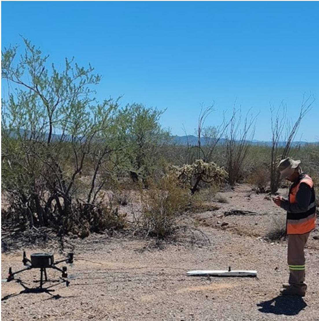
Photo: Drone operator with an airborne magnetometer at Union, Sonora preparing for drone take off.
