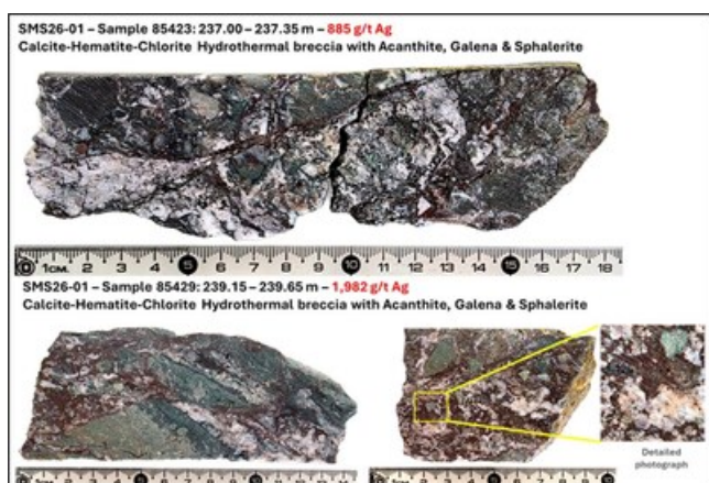
Figure 3: Drill Core Photo Illustration - SMS26-01 High-Grade Samples (CNW Group/GR Silver Mining Ltd.)
