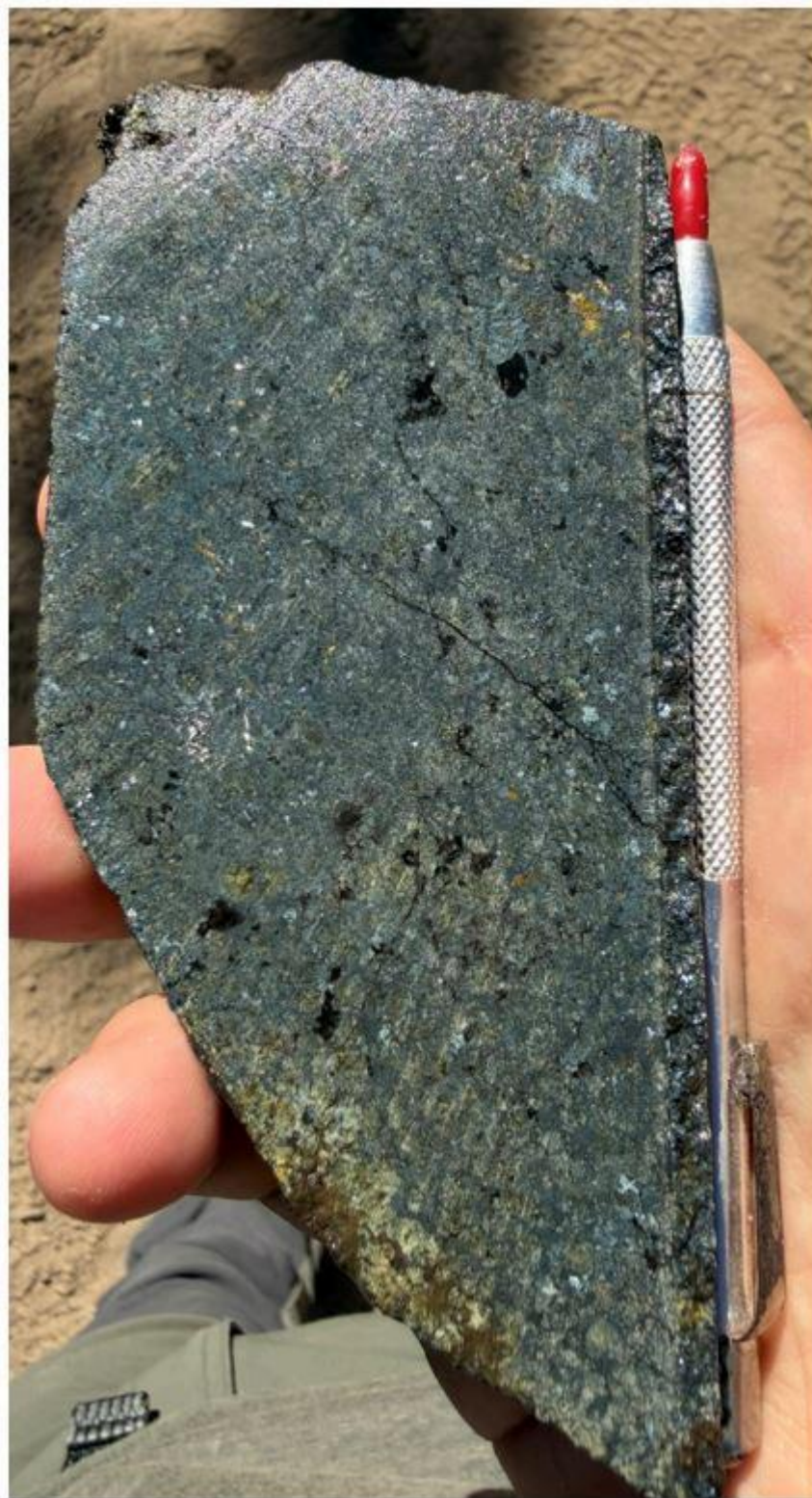
Figure 5. Skarn horizon 3 - Fine grain green-garnet and magnetite skarn with copper sulfides, chalcopyrite and chalcocite.
