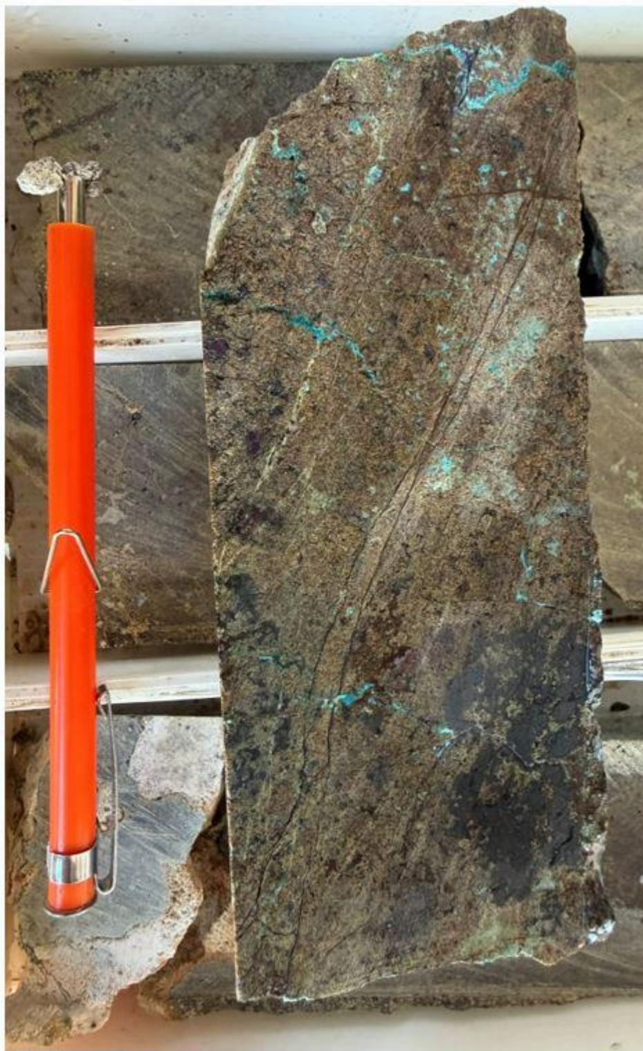
Figure 4. Skarn horizon 2 - Fine grain green garnet skarn, with copper sulfides and oxides along fractures.
