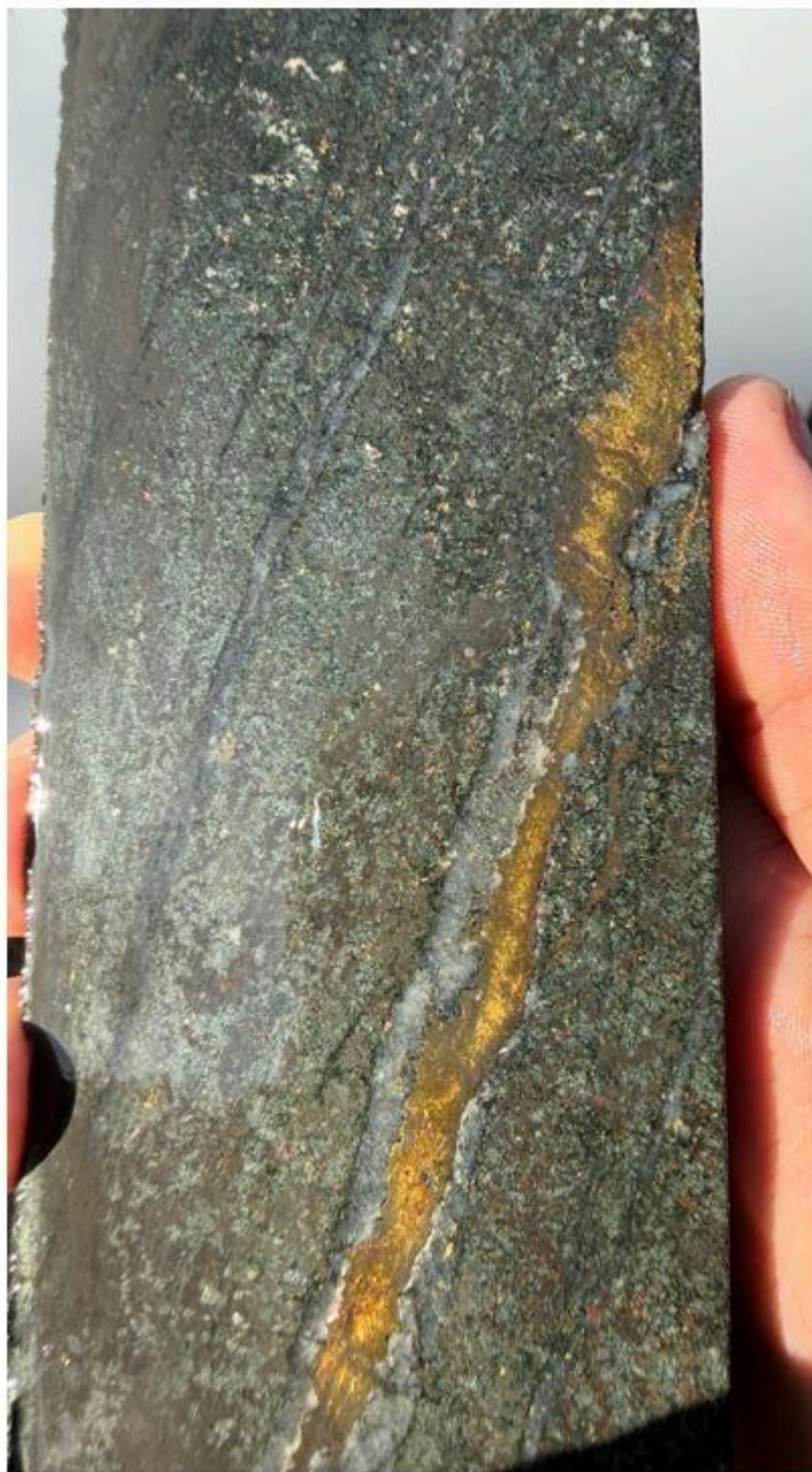
Figure 3. Skarn horizon 1 - Magnetite rich skarn, with chalcopyrite along veins, chalcocite disseminated.
