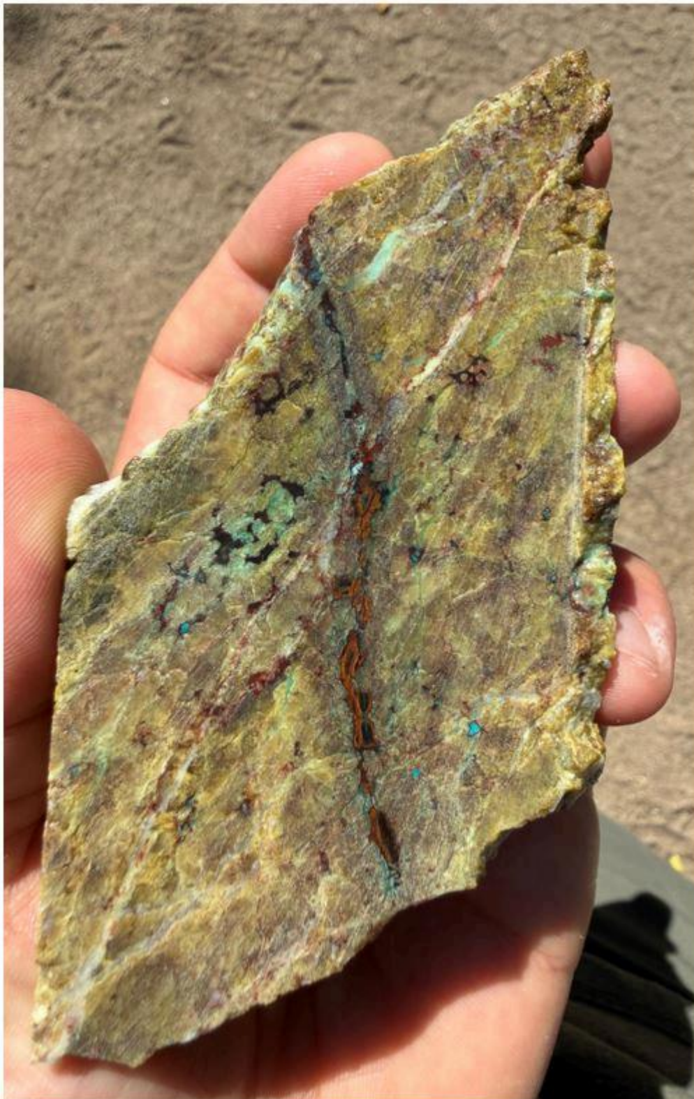
Figure 7. Skarn horizon 5 - Green-garnet skarn with copper sulfides, disseminated and along fractures.
