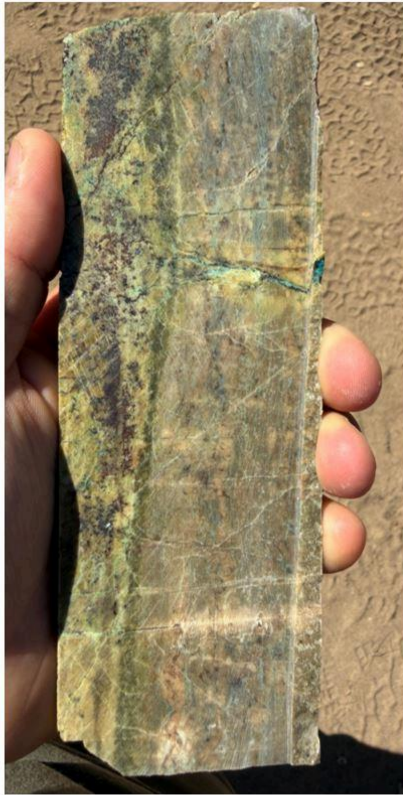
Figure 6. Skarn horizon 4 - Green-garnet skarn with copper and silver sulfides (note the skarn front in the axis of the core sample).
