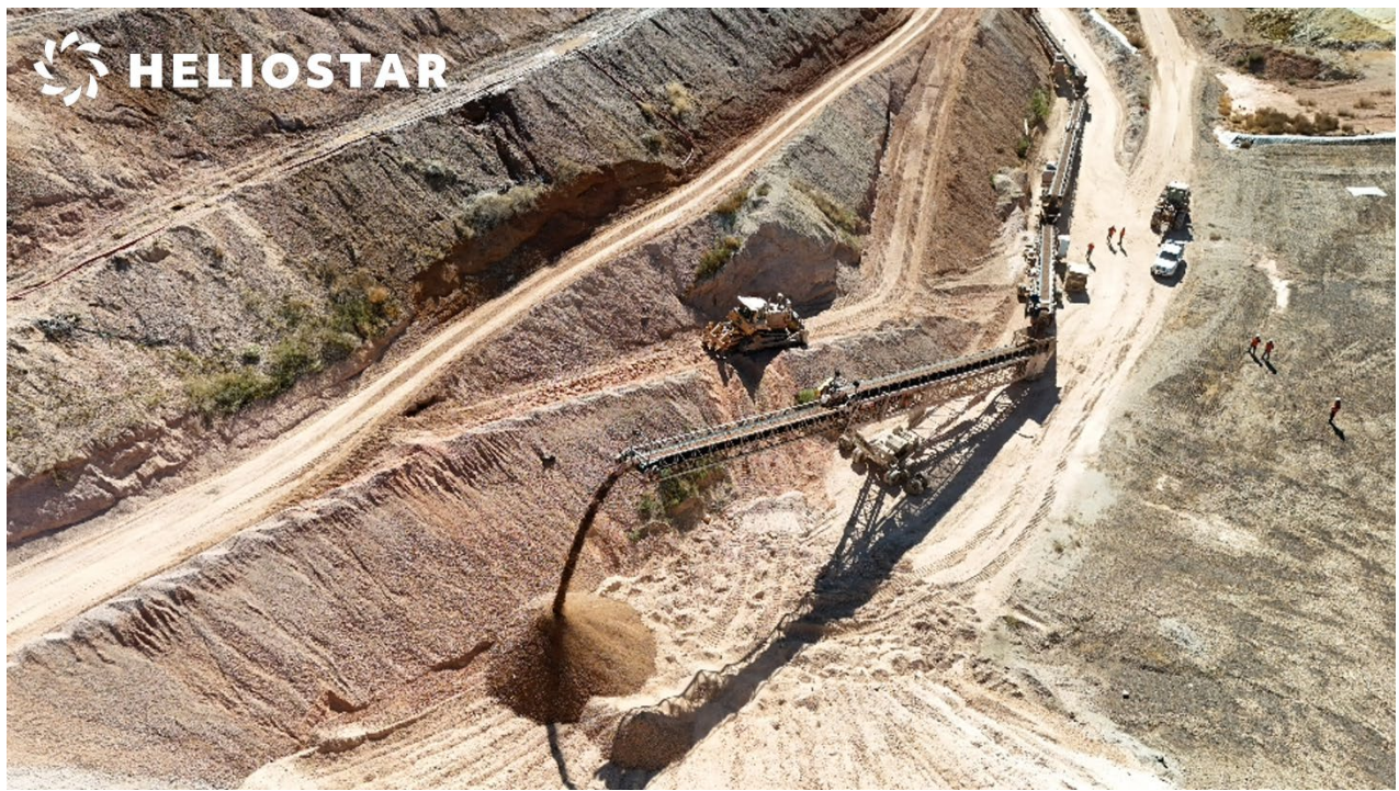
Figure 4: First new ore being conveyed and stacked on the San Agustin leach pad
