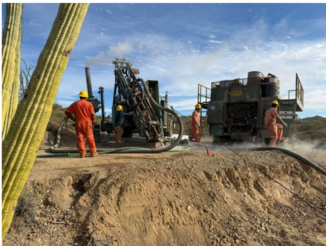
Image 2: Drill mast raised on first prepared pad, RC drilling underway
