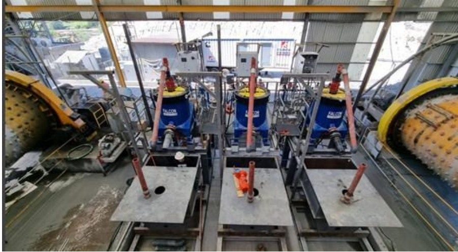
Figure 1. The three new Falcon concentrators installed between the 12 x 8 and 8 x 8 Ball mills.
