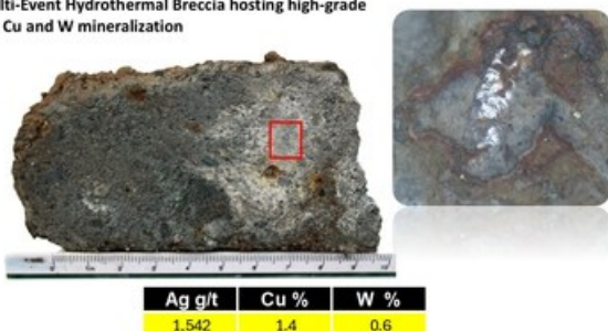
Figure 4 Drill Core Photo Illustration - SMS25-10A “Hydrothermal Breccia” (CNW Group/GR Silver Mining Ltd.)
