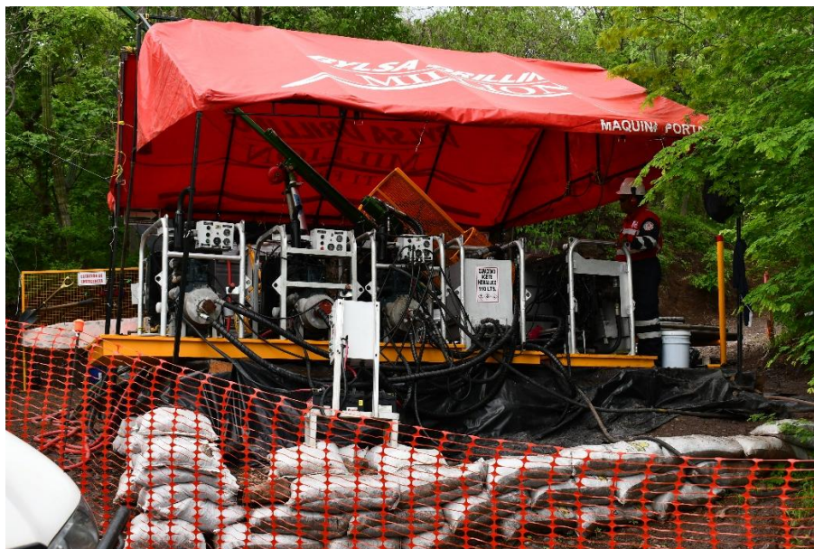
Figure 1. Diamond core drill rig onsite at Alamos Silver Project, Sonora, Mexico.
