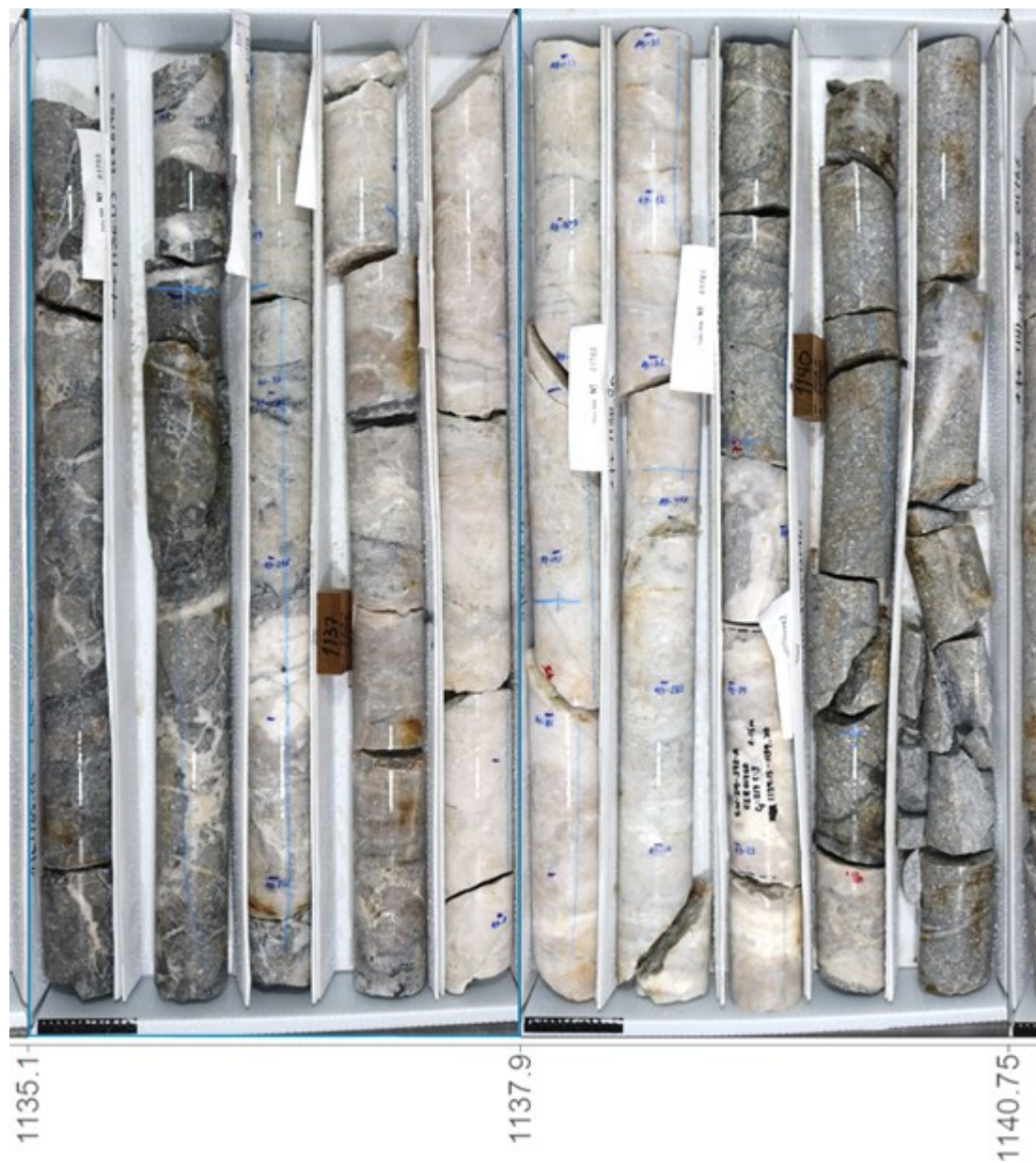
Figure 3: Core Photography of the Navidad Vein with High-Grade Gold and Silver Mineralization detected by XRF Analyzer.
