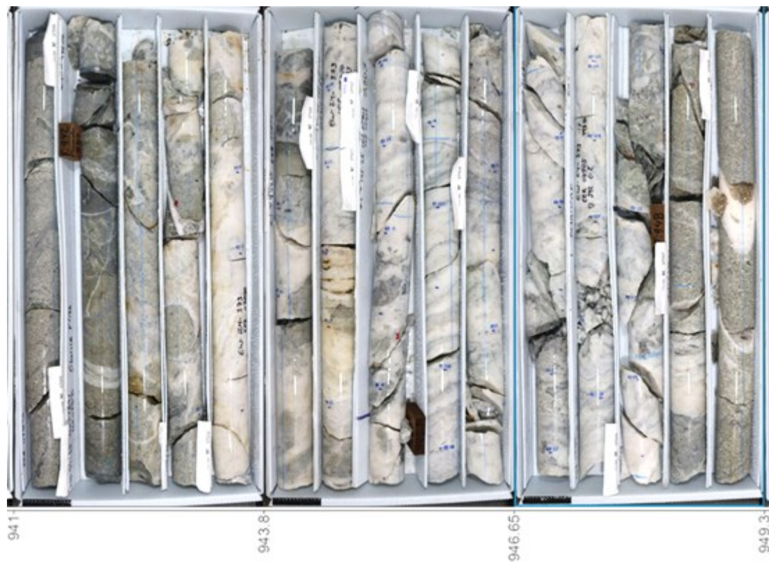
Figure 2: Core Photography of the Winter Vein with High-Grade Gold and Silver Mineralization detected by XRF Analyzer.
