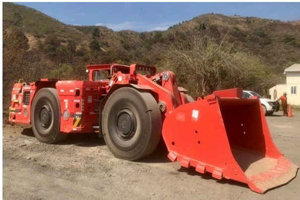
Image 2 – New Scoop Tram at Campo
