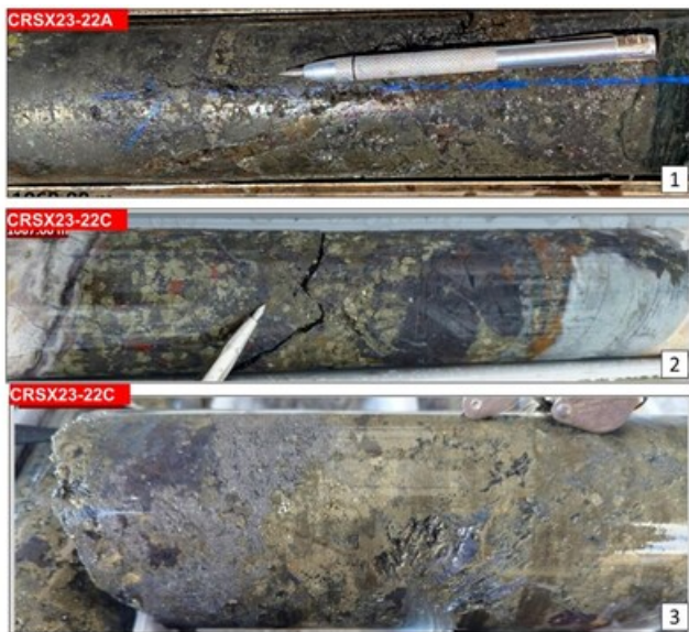
Figure 1: Examples of polymetallic (Au-Ag-Zn) massive sulphide mineralization, Camino Rojo Extension. (CNW Group/Orla Mining Ltd.)
