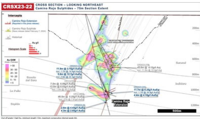
Figure 4: Camino Rojo Extension cross section drill intersection highlights for CRSX23-22 series of drill holes. (CNW Group/Orla Mining Ltd.)
