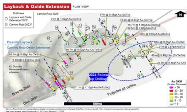
Figure 1: Oxide Layback and Extension Drilling –Drill Intersection Highlights (CNW Group/Orla Mining Ltd.)
