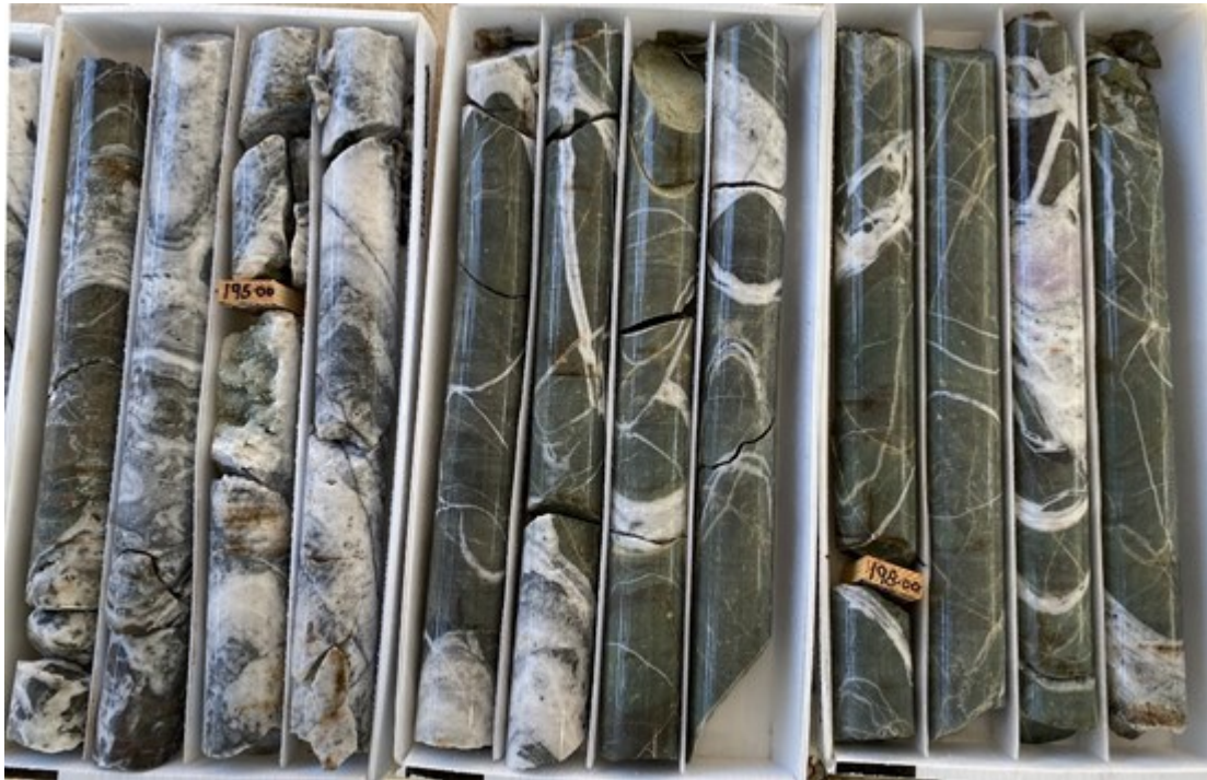
Hole #4 (PV-22-14), 193.55 to 200.0 meters, boxes 87-89, showing 2.5 meter multistage quartz vein on the left with wall rock andesite cut by abundant narrow quartz veins and veinlets.
