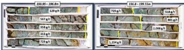
Figure 4: SMS22-10 Select Mineralized Drill Core – Discovery Zone (Ag grades) - Drill Core from 193.95 m to 199.55 m (CNW Group/GR Silver Mining Ltd.)
