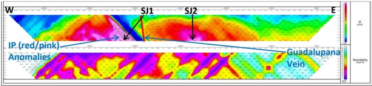
**GEOPHYSICAL CROSS SECTION LOOKING NORTH - DRILL HOLES SJ1 AND SJ2 TARGETING IP ANOMALIES**
