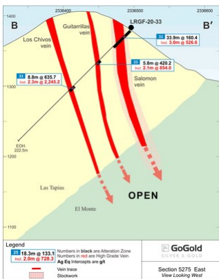
Figure 4: Cross Section – Hole LRGF-21-033 (CNW Group/GoGold Resources Inc.)
