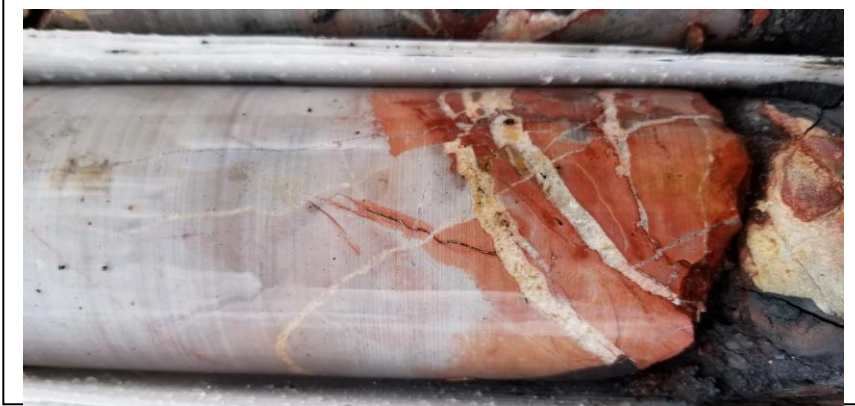
Figure 4. Example of oxidization originating from sulfides in fractures and veins 323m (EA-002).
